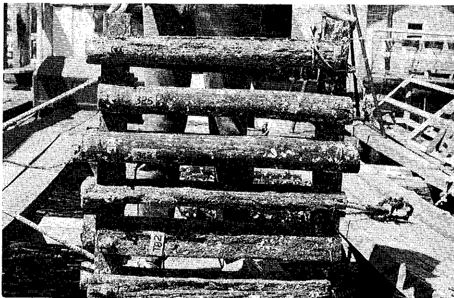
Fig.6. A P5-7 test frame after 26 years in Sydney Harbour. No. 382 (top) = 27kg/m 3 celcure old-E. macrorhyncha with severe attack. No. 325 = 160kg/m 3 high boiling fraction of K55 creosote- E. macrorhyncha with light attack. No. 343 = 320kg/m 3 high boiling fraction of K55 creosote with no attack. No. 367 = 27kg/m 3 Boliden S25-E. macrorhyncha with sapwood destroyed. T82 = untreated sawn turpentine with moderate attack. T74 (bottom) = untreated sawn turpentine with heavy attack
